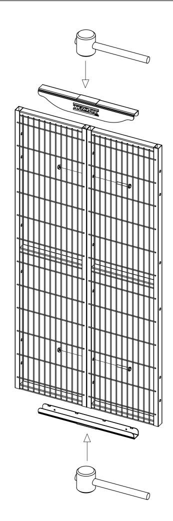
Snapper kit ST30 29500221 Snapper kit ST20 29500231 Includes one upper and one lower profile
