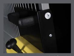
Mount a blind rivet to prevent the Safe Lock from being defeated.
