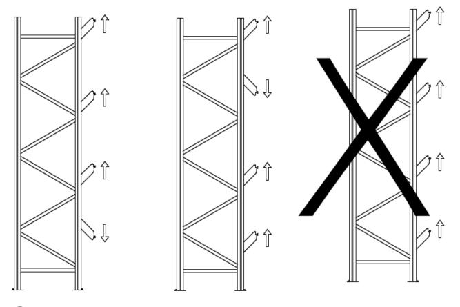
Mounting brackets may be installed angled up or down depending on location of the pallet rack shelving beams. The only requirement is that at least one row of brackets must be mounted opposite of the other rows of mounting brackets.
