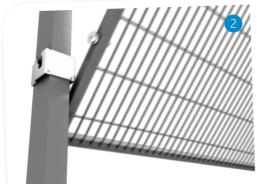
Rapid Fix brackets are more functional. The lower bracket has a slot that the panel hooks into and the upper bracket has a unique locking mechanism that snaps the panel into the correct position. The locking mechanism means that the panels can be
