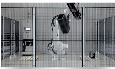
**Real impact test** using an ABB robot with magnetic gripper that ejects a steel tube of 52 kg into the Smart Fix machine guard.
